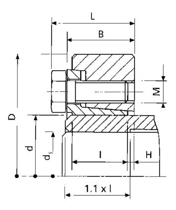
B mm = 26.0 d H8 mm = 50 D mm = 90.0 ds mm = 38 F kN torque = 84 H = 2.5 I mm = 22.0 L mm = 31.5  $\begin{array}{ll} \text{M mm} & = \text{M8} \\ \text{T N m torque} & = 1600 \\ \text{Ts N m bolt tightening torque} = 34 \\ \end{array}$
